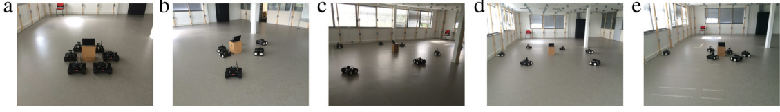
Fig. 4. Deployment of six Wifibot. In (a) shows the initial position of the robots. The spreading phase takes place in (b) and (c). The shrinking phase are represented in (d) and (e).
