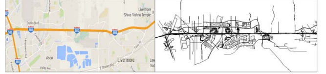
Fig. 4. San Jose (California) urban area captured from Google Maps (left) and exported to a VANET network topology by using MOVE/SUMO (right).
