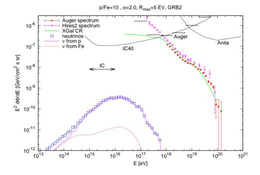
Figure 4: Mixed composition (p–Fe) scenario with source spectral index  $\alpha = 2.0$ and  $E_{max} = 5 Z$  EeV. Indicated are the propagated CR spectrum, the resulting (all flavor) neutrino fluxes and the separate contributions from p and Fe primaries.
