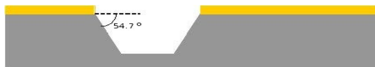
Figure 3. Si (100) showing characteristic V anisotropic etch of the walls forming an angle of 54.7^\circ with respect to the main surface.
