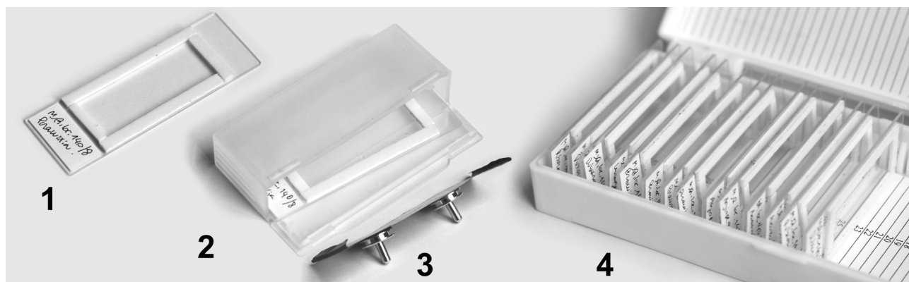
FIGURES 1–4. Silk samplers, boxes and specimen holder. 1, Silk sampler; 2, Small portable specimen box; 3, Specimen holder for SEM examination; 4, Slide box with silk samplers, for long-term storage.
