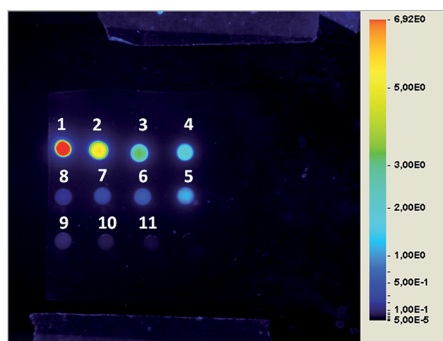
Fig. 2 NIRF imaging of glucan particles diluted in PBS at different concentrations ranging from 18 \times 10^6 GPs per μL to 3.5 \times 10^4 GPs per μL. (1) 18 \times 10^6 GPs per μL, (2) 9 \times 10^6 GPs per μL, (3) 4.5 \times 10^6 GPs per μL, (4) 2.2 \times 10^6 GPs per μL, (5) 1.1 \times 10^6 GPs per μL, (6) 5 \times 10^5 GPs per μL, (7) 2.5 \times 10^5 GPs per μL, (8) 1.25 \times 10^5 GPs per μL, (9) 7 \times 10^4 GPs per μL, (10) 3.5 \times 10^4 GPs per μL. Sample 11 corresponded to PBS (control).
