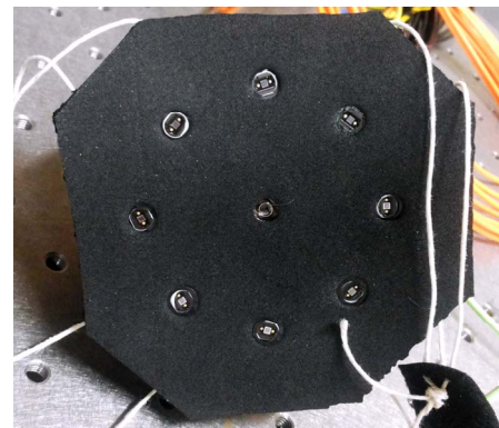
Figure 2. Picture of the designed probe. The laser source, in the center, is surrounded by the 8 SiPM channels
