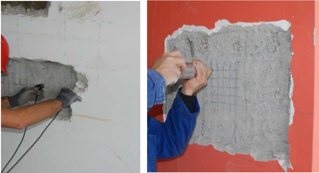
Figure 4. Example of ultra-sonic and sclerometric tests.
