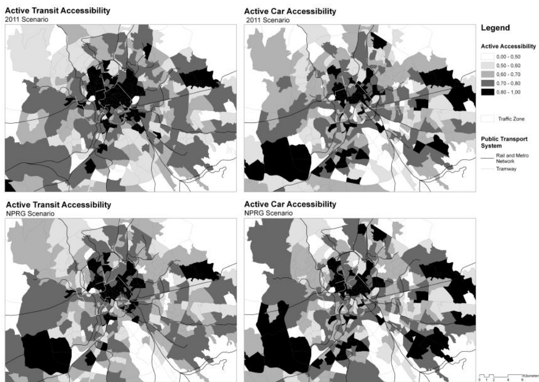
Figure 3. GraBAM outputs: comparing car and transit active accessibility in different scenario: 2011 scenario vs. NPRG scenario (i.e. the Master Plan of Rome).
