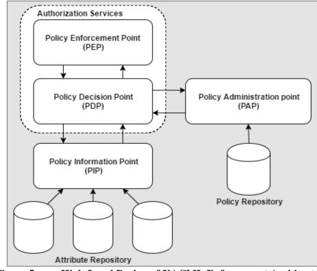
Figure 5 High-Level Design of XACML Enforcement Architecture
