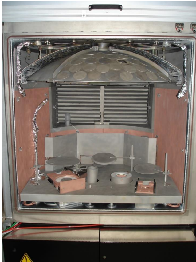
Figure 4.2 - PIAD deposition plant APS 904 (Leybold Optics) used for all depositions of the 1DPC. Courtesy of Fraunhofer-IOF.
