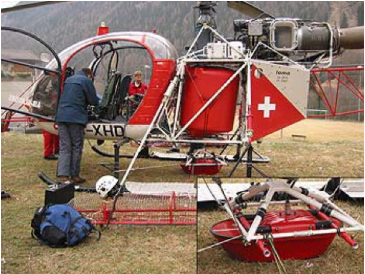
Fig. 10 – GPR system mounted on an airborne platform (from the Radarteam Sweden AB web-site)
