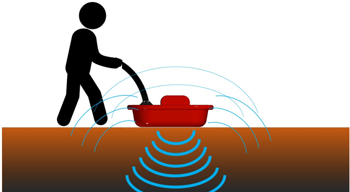
Fig. 1 – GPR radiates energy into the ground normally with reduced back-propagation toward operator.
