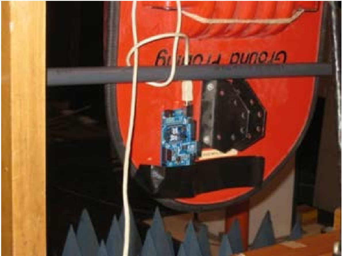
Fig. 13 – XBee transceiver on the top of the antenna.
