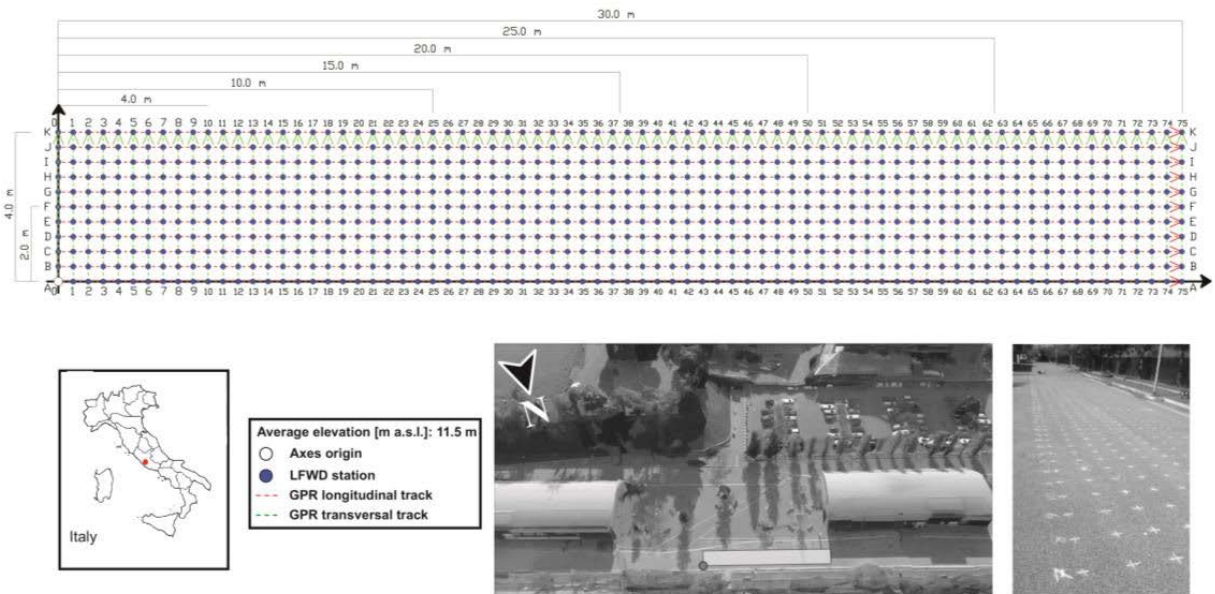
Fig. 18 – Test site for data acquisition carried out over a 4m×30m square regular grid mesh of 836 nodes.
