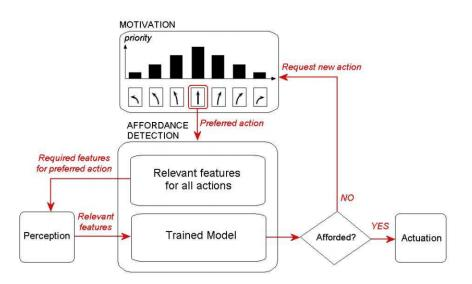
Figure 3.5. Robot control system exploiting affordances, from Ugur et al. [142].
