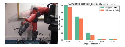
Figure 8.5. Results on controlling a Baxter robot with a steady-state control policy. We learn a dynamics model and compute a policy to move the robot manipulator from state  $s_0$  to  $s_T$ .
