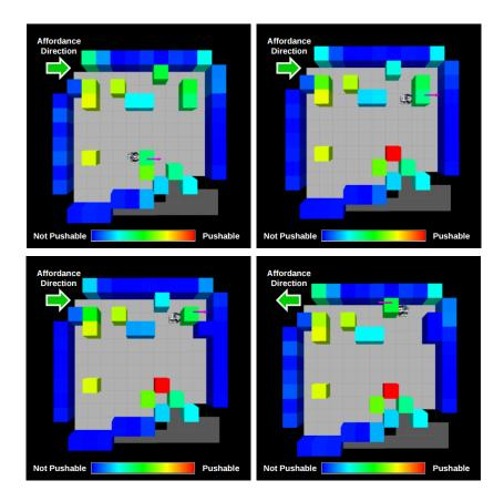
Figure 3.6. Heatmap representing the affordability of the "push" action during a sequence of robot manipulation steps in a grid world, from Kim and Sukhatme [67].
