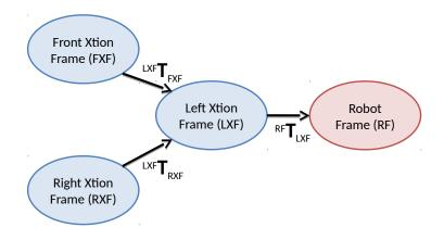
Figure 4.6. Sensor transformation tree generated at the end of the calibration procedure for a robot equipped with 3 depth cameras.
