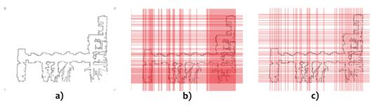
Figure 6.3. Steps of the construction of the A-Grid [20], given a metric map.
