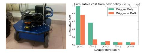
Figure 8.4. Results for controlling a Videre Erratic differential-drive mobile robot in open-loop.
