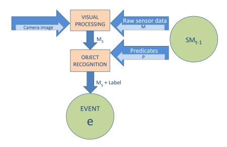
Figure 6.2. Event (label and subset of sensor data) generated through autonomous object recognition.
