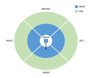
Figure 6.4. Example of qualitative spatial relations. Here, relative directions are computed against the intrinsic normal vector of an object, while distances are highlighted with circles of different colors.
