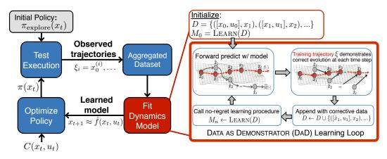
Figure 8.1. (Left) DAgger System Identification for model learning and control. (Right) DAD improves the multi-step prediction performance of learned dynamics models.
