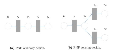
Figure 2.4. Ordinary and sensing actions in a Petri Net Plan.
