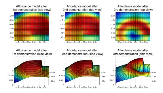
Figure 5.4. Spatio-temporal affordance of a following task, at a given time t, learned with increasing number of expert demonstrations. Here, the target is located at the origin and the plots represent the probability density function of a pose to afford the task. The plots, whose coordinates are expressed in meters, show that the model is able to represent both minimum and maximum distances from the target, in accordance with the data provided as demonstrations.
