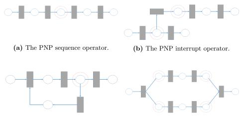
(c) The PNP loop operator. It can be (d) The PNP fork and join operators. used to define definite or indefinite loops.
