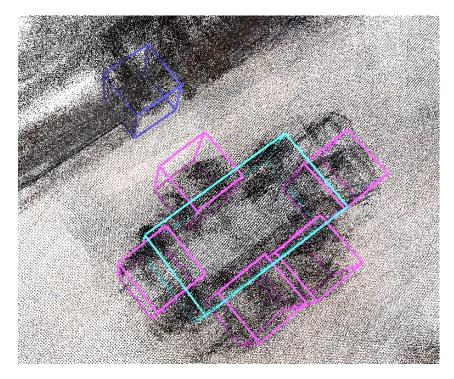
Figure 4.9. Detail of the example dataset acquired in the RIF of Peccioli. The image shows a table and chairs with their associated bounding boxes. RGB information is intentionally omitted and resolution is reduced for a better visualization of the bounding boxes.
