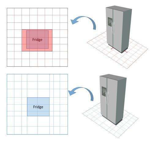
Figure 4.3. Example of structural bias of a semantic map with fixed and adaptive grids.
