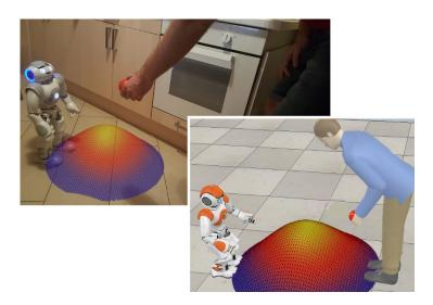
Figure 7.5. Human-robot handover with  $\pi$ -STAM both in real world and simulation.
