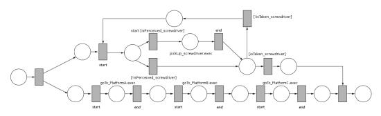
Figure 6.5. Example of PNP for visiting platforms and picking-up a screwdriver.
