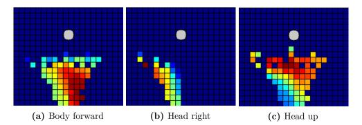
Figure 7.9. Heat-map of the spatial affordance distribution generated by  $\pi$ -STAM (after 3 iterations) for the body forward, head right and head up actions. The initial distribution was composed of states located at a distance between 45cm and 60cm in front of the target. Each cell of the grid has a size of approximately 5cm. Red colors represent high affordance values in the cell, while blue colors represent low values.
