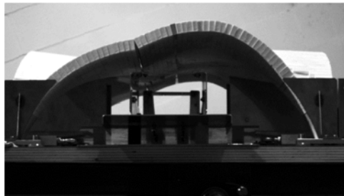
Figure 4-30. Tilting test: deformed shape (seismic direction = 0°) with K_n = 1, K_t = 0.1, 0.4, 1 MPa/mm (considering UL)
