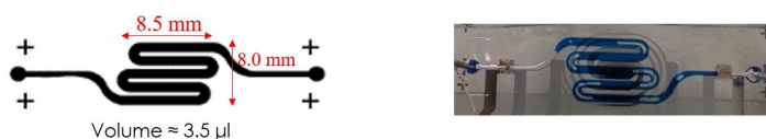
Figure 3.18. Serpentine shaped microfluidic channel (left), non-correct filling occurred during the fabrication (right).
