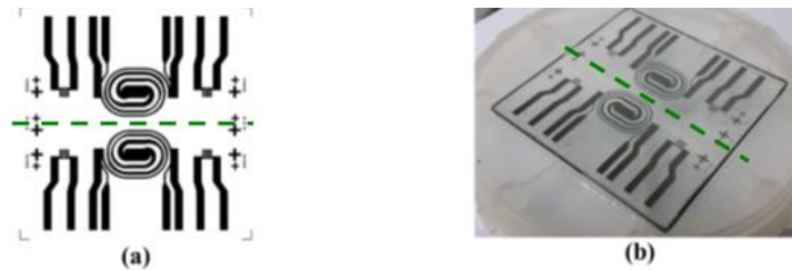
Figure 2.13. (a) Heater mask (mask #5); (b) Fabricated heaters
