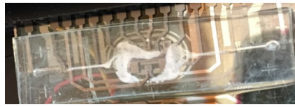
Figure 3.10. Fabricated microfluidic network aligned with the DARWIN'S device: air bubbles expansion during the PCR heating.
