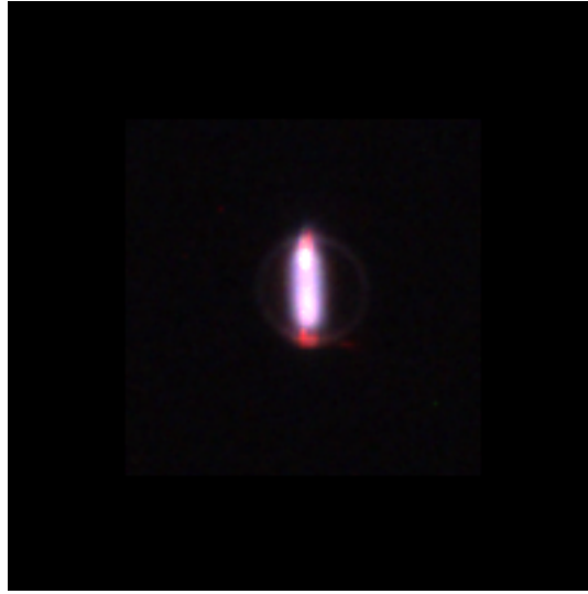
Figure 6.8. Typical picture taken from 90^\circ our Thomson scattering diagnostics. By dividing the length of gas-jet diameter by the number of pixels constituting it in the image, it is possible to retrieve the CCD camera calibration. The plasma channel created by the laser propagation in the gas is visible as well.
