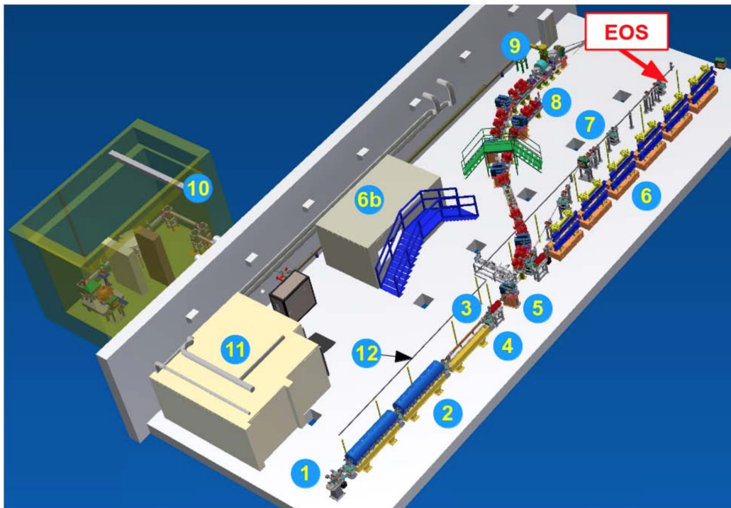
Figure 2.1. SPARC_LAB layout. From bottom: the electron-gun (1) followed by the three TW accelerating sections (2). A THz station (3), that will host PWFA experiments, is located before the three quadrupoles and a RFD (4) for diagnostics and matching; these are then followed by the first dipole (5). Four beamlines follows the dipole, devoted to FEL physics (6) both in SASE and seeded (6b) schemes, beam diagnostics (7) based on EOS and THz radiation, plasma acceleration by LWFA (8), and X-rays production in the Thomson interaction chamber (9) by colliding the electron beam with the FLAME laser (10). The EOS laser comes from the photo-cathode laser room (11) and is delivered to the EOS station by using the EOS transfer line (12). [60]
