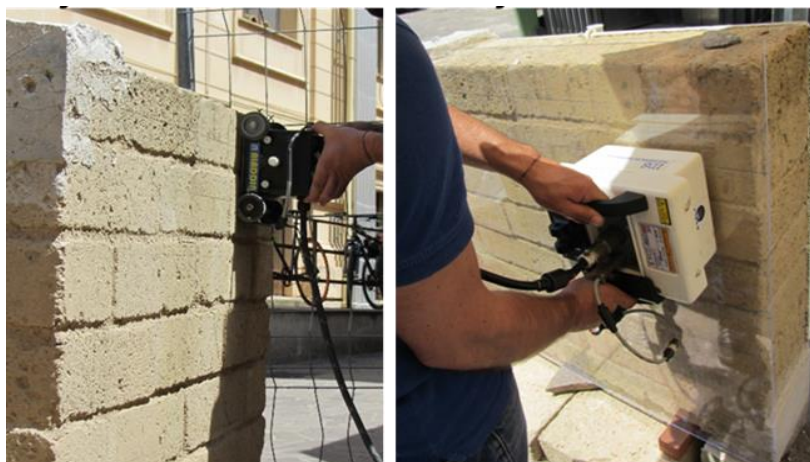
Figure 4.6: Images of the 2000 (a) and 900 (b) MHz antennas on the tuff sample.
