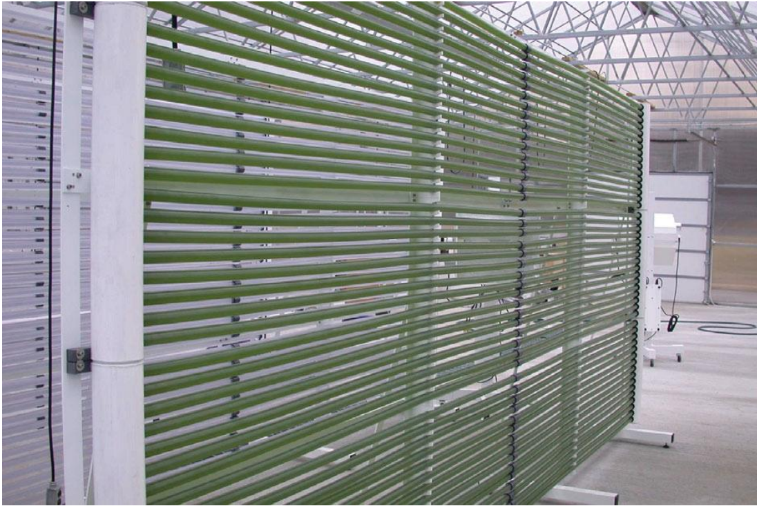
Figure 2.5 – An example of photobioreactor (tubular shape).
