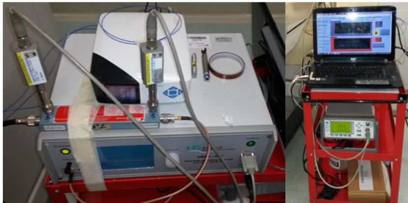
Figure 2.3.6 Experimental setup for MTA under CT control: MiW generator, directional coupler, and fiber optic thermometer (left); power meter and laptop with a dedicated LabVIEW program for procedure control and data storage.
