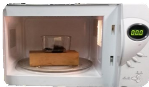
Figure 2.3.3 Experimental setup for carbonization of restricted samples of biological tissue.
