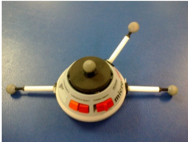
Figure 2.3.2: The microFET2® Hand Held Dynamometer equipped with passive motion capture markers.
