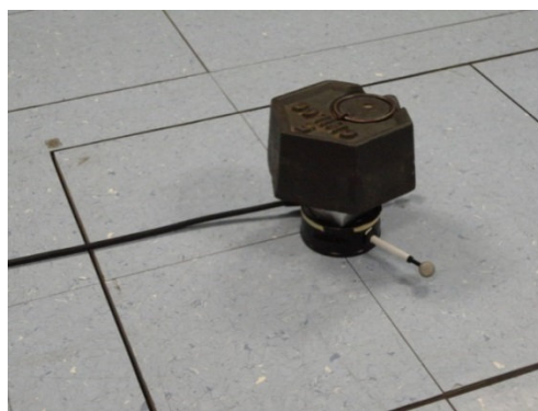
Figure 2.4.5: Testing of the load cell by applying a known load in series to the load cell and the force plate.
