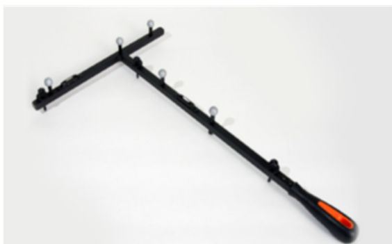
Figure 2.4.6: T-shaped calibration wand for the Vicon MX system.
