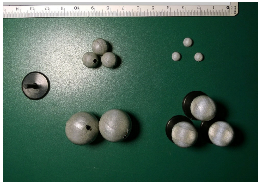
Figure 1.3.3b: IR reflective markers for motion capture.
