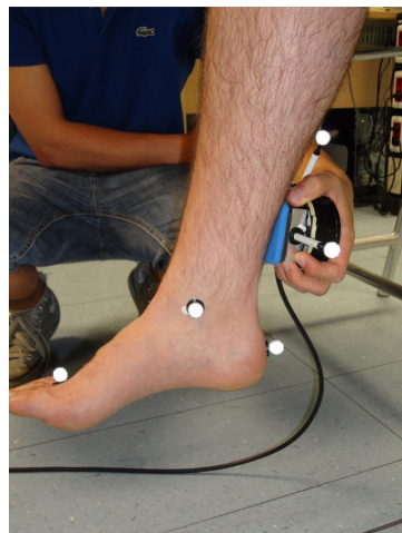
Figure 2.4.10: HHD placement for knee flexion trials.
