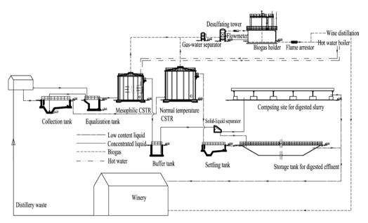
Fig. 1 – The process flowchart of the biogas plant.
