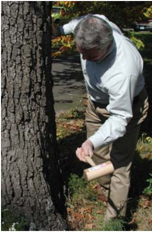
Bruce Spaman, Superintendent of Parks and Tree Warden for the Town of Greenwich, using a mallet to listen for the soundness of the tree to test for decay.
