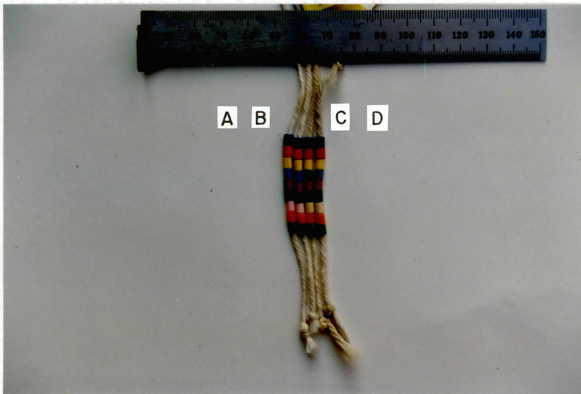
Figure 11. --Comparison of unexposed and sunlight-exposed color bands. New color bands (A) began color changes within one week of exposure in full sunlight (B). After 30 days of exposure, PINK bands had shifted in color to a faded yellow (C), and after 90 days of exposure, PINK bands had lost all color and were an off-white.
