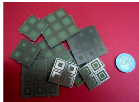
Fig. 32 – Prototypes of chipless RFID tags of different dimensions (2x2 and 3x3 unit cells). Figure reproduced with permission [47]. Copyright 2013, IEEE.
