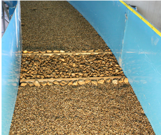
Figure 4. Picture of the experimental apparatus illustrating the modelled block ramp 4 (view from downstream).
