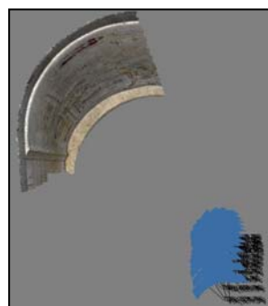
Figure 12 – Photogrammetric DPC left first third area and camera locations in right lateral row.
