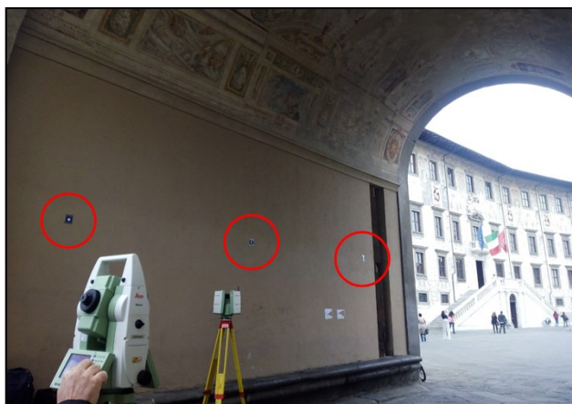
Figure 17 – View of the survey of Leica HDS 3'' targets (circled in red colour) and location of "Leica C-10" TLS.
