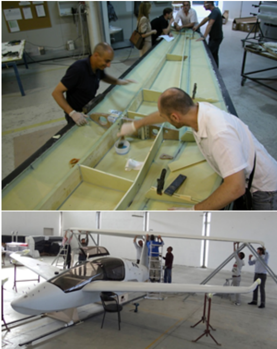
Figure 25. Full scale prototype of the light amphibious PrandtlPlane: rear wing manufacturing and preliminary assembly
