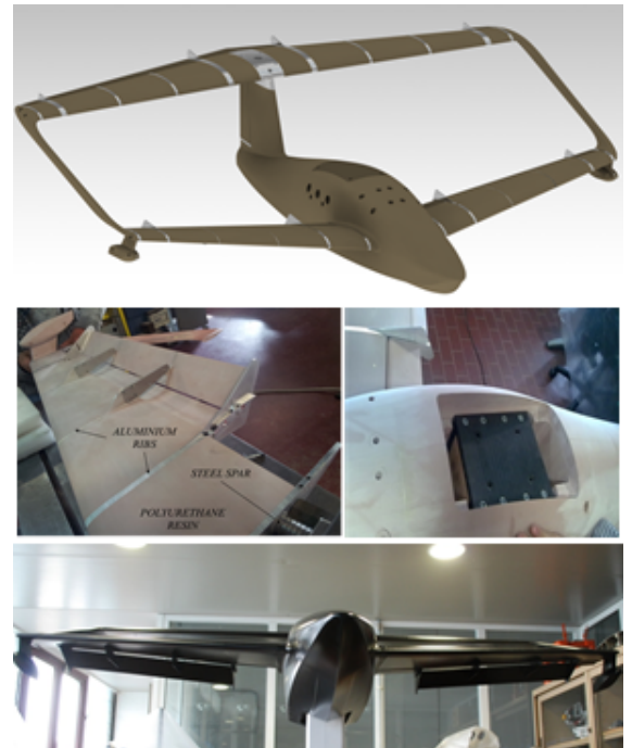
Figure 22. Some details on the manufacturing of the 1/4 scaled model for the wind tunnel tests
