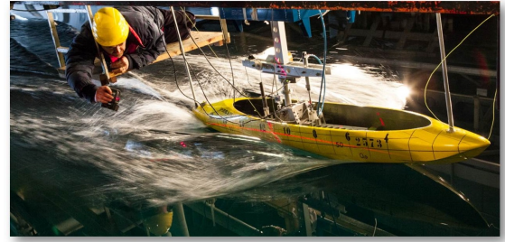
Figure 16. Stability test at the towing tank facility of CNR-INSEAN in Rome (this photo was the winner of photographic competition in Italy to celebrate the 90 years from the foundation of CNR)
