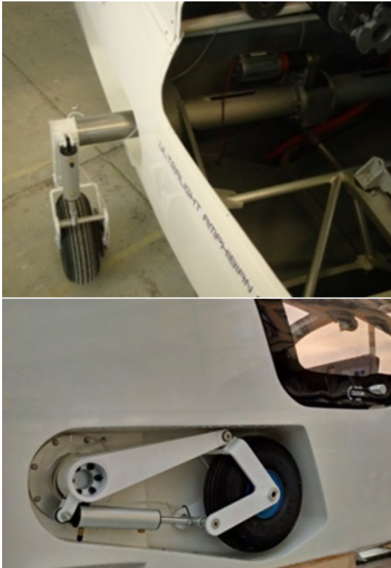
Figure 30. Main undercarriage of the amphibian (external shield missing)
