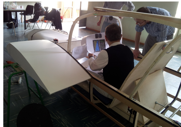
Figure 6. Visibility and ergonomic tests on a full-scale maquette (ISIA, Florence)
