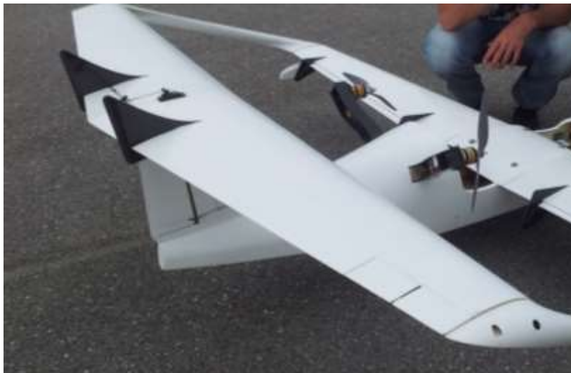
Figure 33. Rear fences on the flying model.
