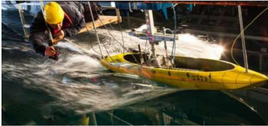
Fig. 3 Towing tank tests on the 1/3 scaled model of the hull at CNR-INSEAN in Rome
