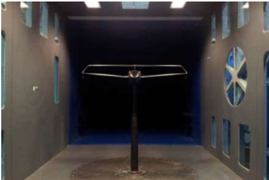
Fig. 4 Wind tunnel tests on IDINTOS 1/4 scaled model
