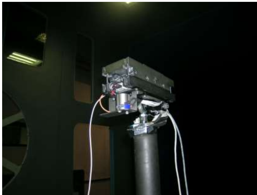
Fig. 7 The 6-components balance and the strut
