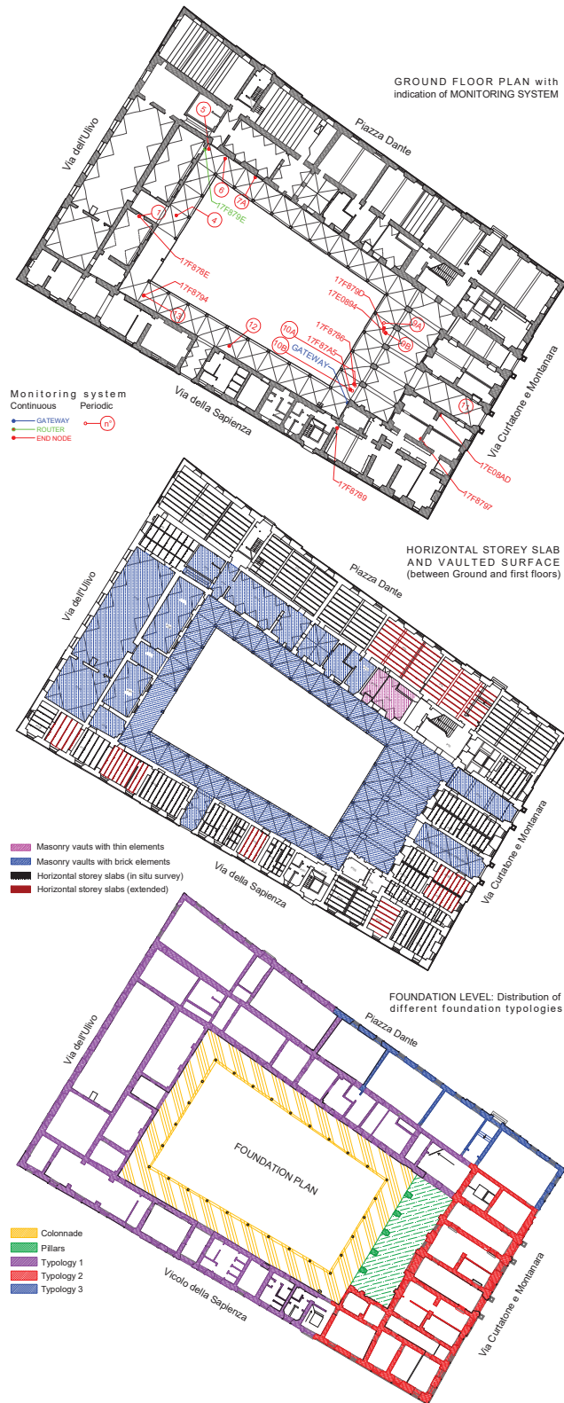
Figure 3: Distribution of the floor slabs and types on the building's ground floor, Foundation plan, different typologies evidenced and ground floor plan with indication of monitoring points.
