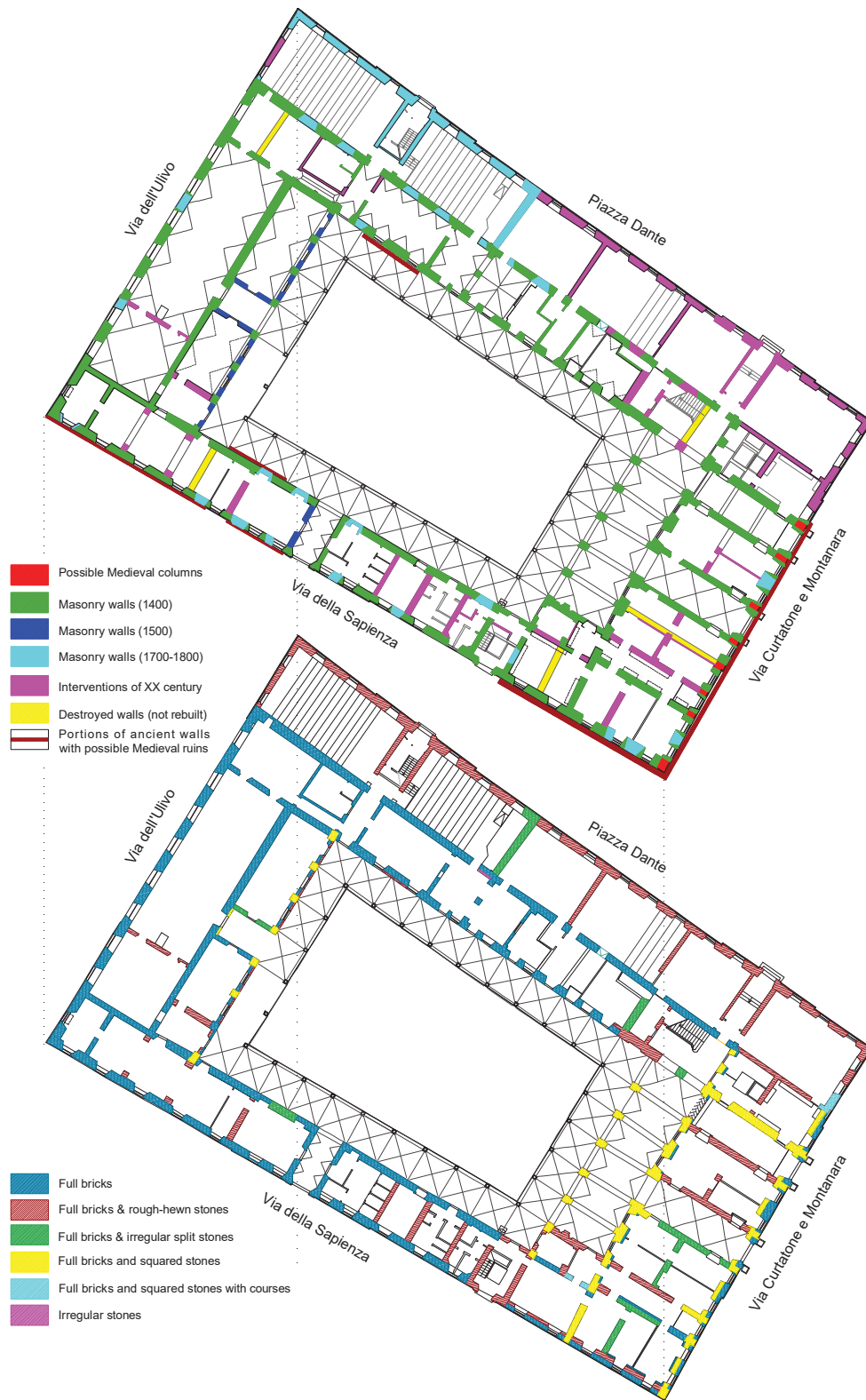
Figure 2: Hypothesis of the evolutive development of the building and plan of ground floor with indications of the various types of masonry.
