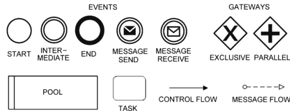
471 Figure 3. Basic BPMN elements: events, gateways, pool, task, flows.
