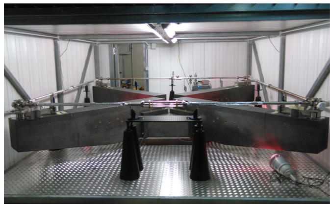
Figure 3 – GINGERino apparatus in the underground Gran Sasso INFN laboratories (color on line).
