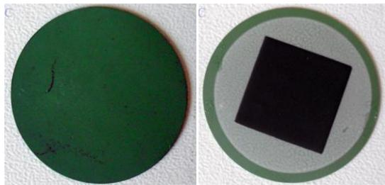
Figure 7 (left) SOFC anode, (right) SOFC cathode
