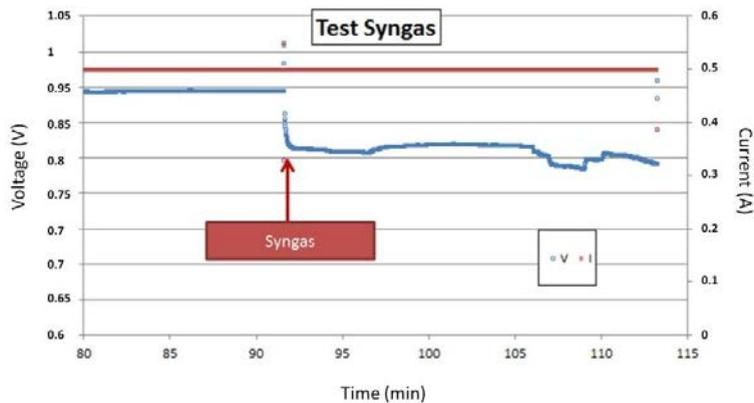
Figure 8: Constant load SOFC performance under syngas.
