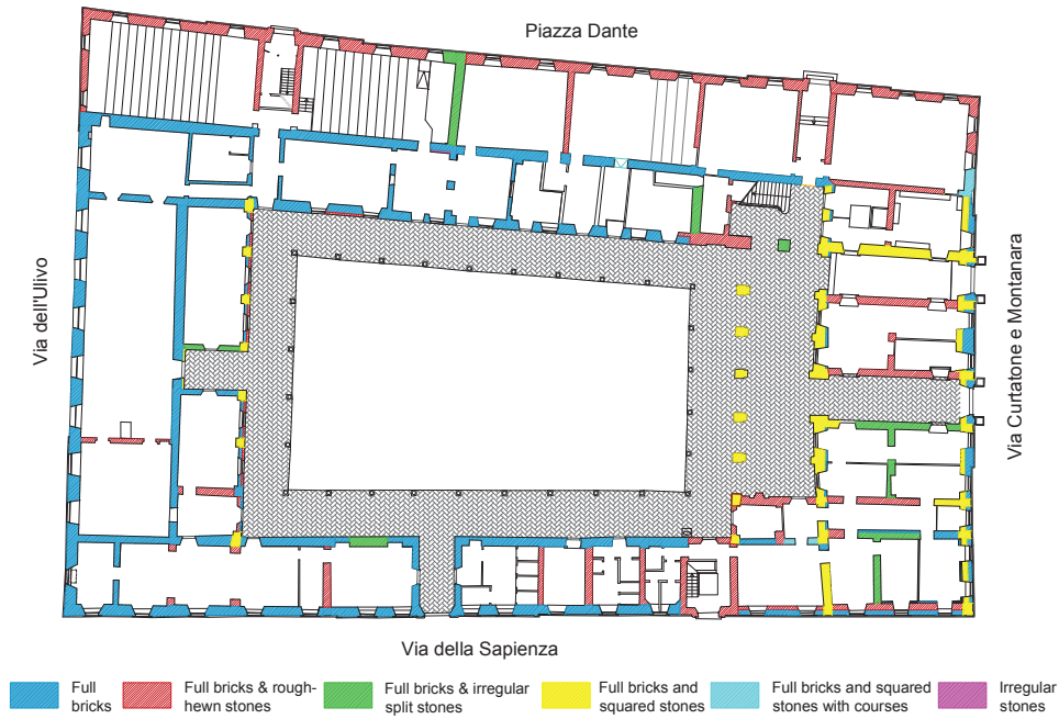
Figure 5: Plan of ground floor with indications of the various types of masonry
