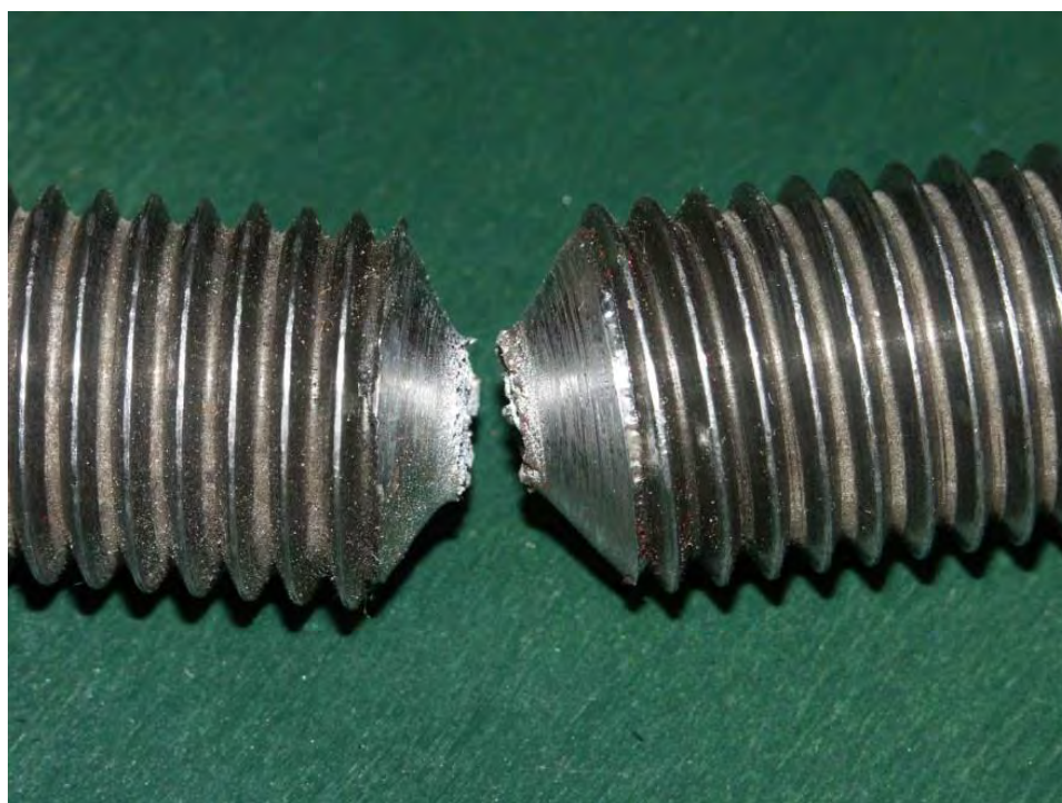
Figure 7 Detail of the calibrated bar (before and after breaking)
