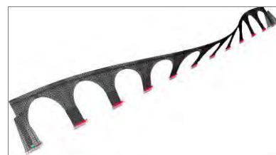
Figure 57 The third mode shape of the structure
