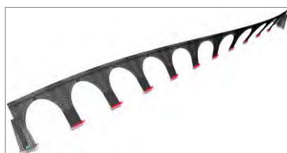
Figure 56 The second mode shape of the structure
