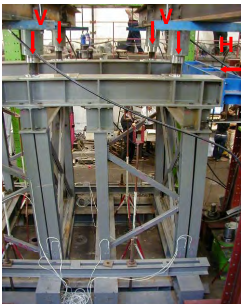
Figure 8 Testing pier P-6 ancillary support
