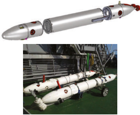
Fig. 4. The Typhoon CAD design and its final built versions on the NATO Alliance RV (CommsNet13).
