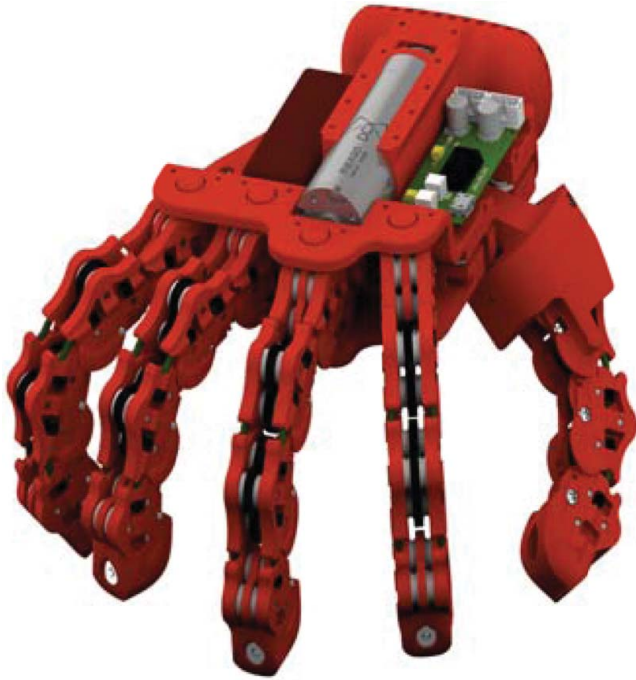
FIG. 1. A preliminary prototype of synergy-inspired hand developed at the Italian Institute of Technology and University of Pisa, Italy.
