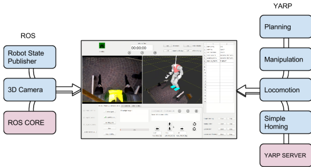
Figure 3: The usage of YARP and ROS in the communication layer
