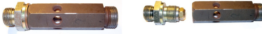
Figure 4. External mixer with the nozzle. Shown on the right are the two components before assembly, and on the left are the nozzle and mixer assembled.
