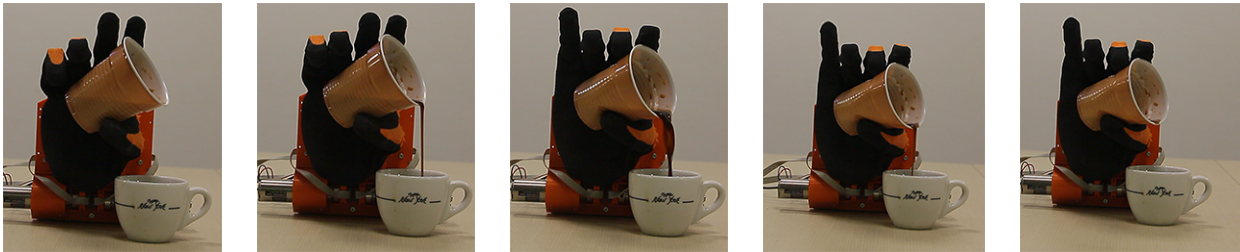
Fig. 14. In-hand manipulation: pouring coffee from a cup, photo-sequence (from left to right).
