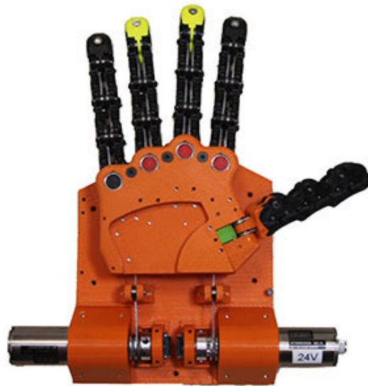
Fig. 1. Prototype of the Pisa/IIT SoftHand+, an evolution of the Pisa/IIT SoftHand with an additional DOA, powered by a friction based transmission.
