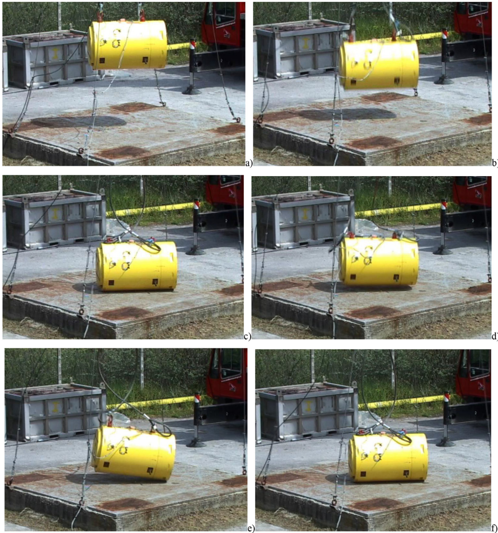
Fig. 3. Sequence of the horizontal drop test execution (Lo Frano et al., 2014).
