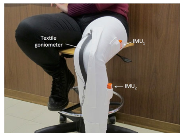
Figure 8 Dynamic test set-up: double layer KPF goniometer applied to a band for the detection of knee flexion/extension; two IMUs are fixed to the thigh and on the calf in order to provide a reference measurement of the knee flexion/extension angle.
