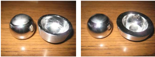
Figure 1 Worn MoM hip implants
