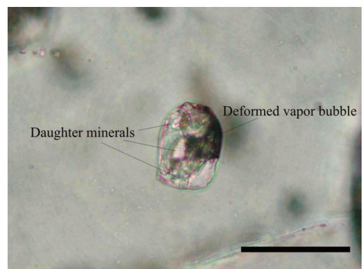
Figure 1. Microphotographs of multiphase fluid inclusion in endoskarn xenoliths. Plane polarized light. Scale bar 40 \mu\text{m} .
