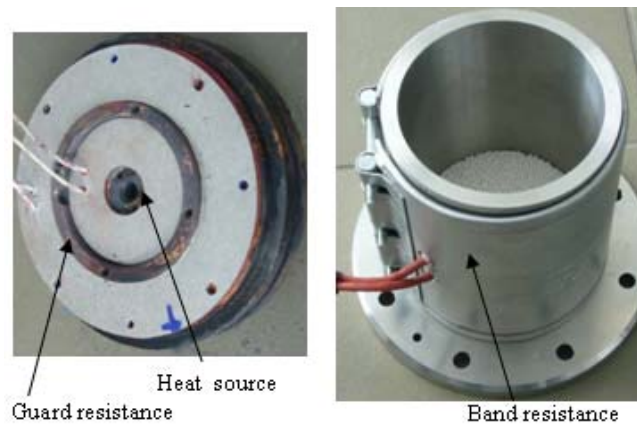
Figure 2. Heating source: electrical resistances.
