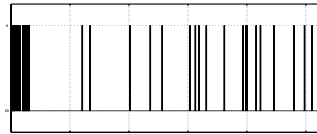
Figure 3. Value of the input event vector u = (a_1, \dots, a_{50}, b_1, \dots, b_{50}, c_1, \dots, c_{50}, d_{1,1}, \dots, d_{50,50}) , representing the activity of a malicious user, including creation of a file in the system's folder of host 33, launch of an application on the same host, opening a large number of connections from host 33 to host 50, remotely start of an application on host 50, and opening of a large number of connections from host 50 to host 1.
