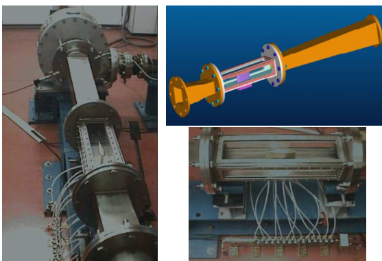
Figure 3 The Cavitating Pump Rotordynamic Test Facility in ALTA S.p.A. in the water tunnel configuration used for tests on hydrofoils ([21]).
