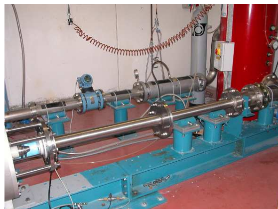
Figure 2 The Cavitating Pump Rotordynamic Test Facility in ALTA S.p.A. in the configuration used for tests on turbopumps ([22]).
