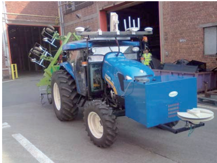
Fig. 2. Pictures of the very first prototype of the machine for precision weed control.
