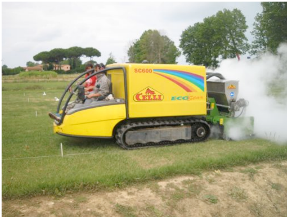
FIGURE 1: Operative machines for flaming and steaming applied on turf.
