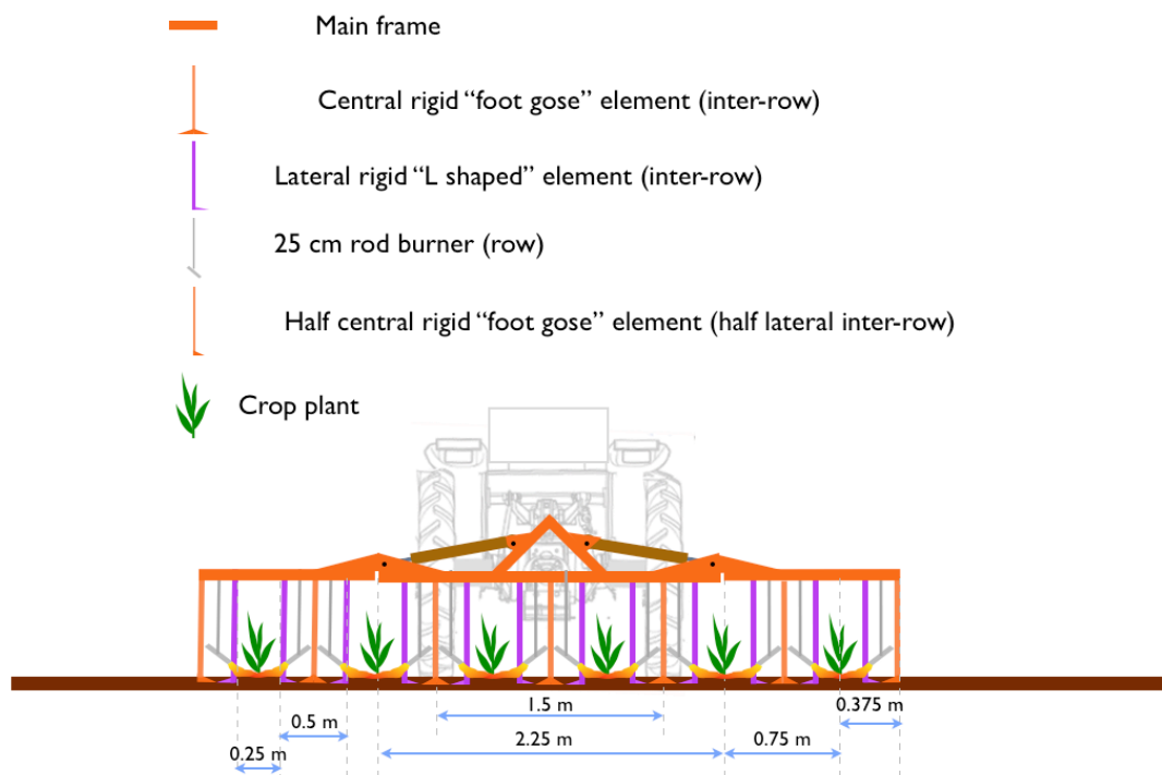
FIGURE 1: Simplified scheme of the operative machines linked at the autonomous ground mobile unit
